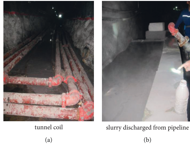
FIGURE 5: Experimental scene of large gravity flow. (a) Tunnel coil. (b) Slurry discharged from pipeline.
