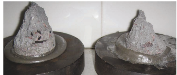
FIGURE 24: The failure of specimens under dynamic pressure.
