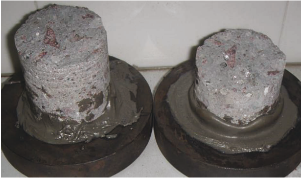
FIGURE 26: The failure of specimens under dynamic tensile.
