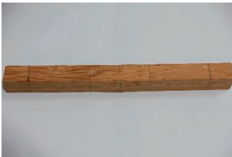
FIGURE 4: Failure mode of bending specimen.
