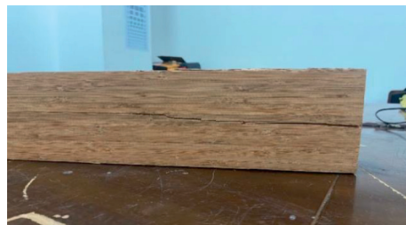
FIGURE 12: Failure mode of shear beam.
