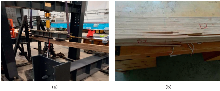
FIGURE 11: Failure mode of bending beam. (a) Groups A and B. (b) Group C and D.
