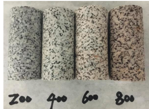
FIGURE 3: Granite specimens after high-temperature heating treatment.
