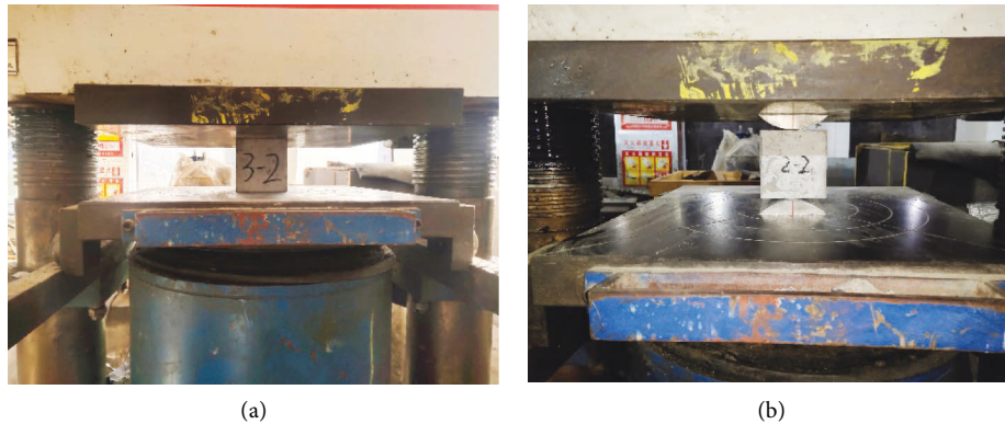
FIGURE 4: Mechanical property test. (a) Compressive strength test and (b) splitting tensile strength test.
