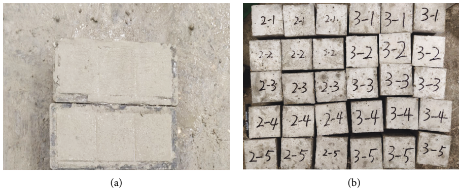
FIGURE 2: Specimen preparation. (a) Specimen pouring and (b) specimen curing for 28 days.
