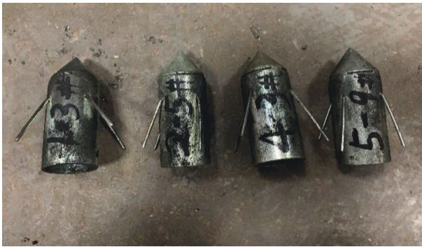
FIGURE 16: Measuring point device after recovery.
