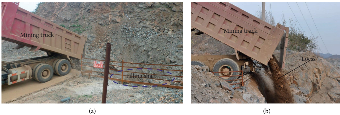
FIGURE 4: The filling process by mining truck. (a) Waste rock filling. (b) Loess filling.
