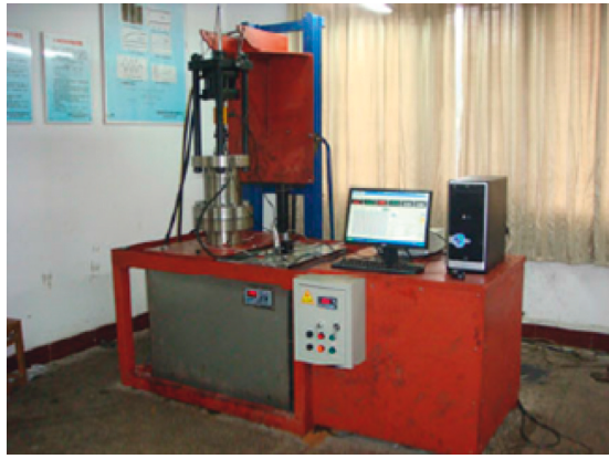
FIGURE 1: Triaxial stress thermal-hydro-mechanical coal containing gas permeameter [20].
