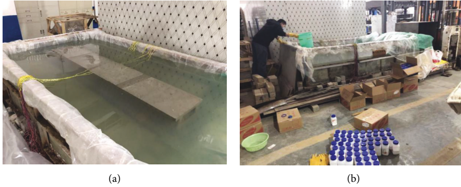
FIGURE 3: Immersion test of the model beam. (a) Immersion model beam. (b) 10% \text{Na}_2\text{SO}_4 solution configuration.
