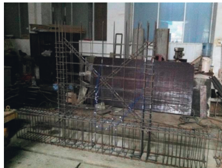
FIGURE 1: Reinforcement details and the actual model of HDLSW. (a) Reinforcement details of HDLSW. (b) Actual model of HDLSW.
