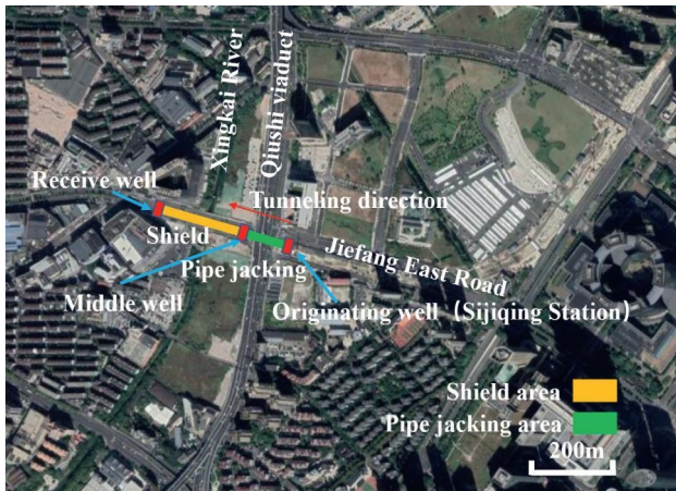
FIGURE 1: Tunnel location plan.
