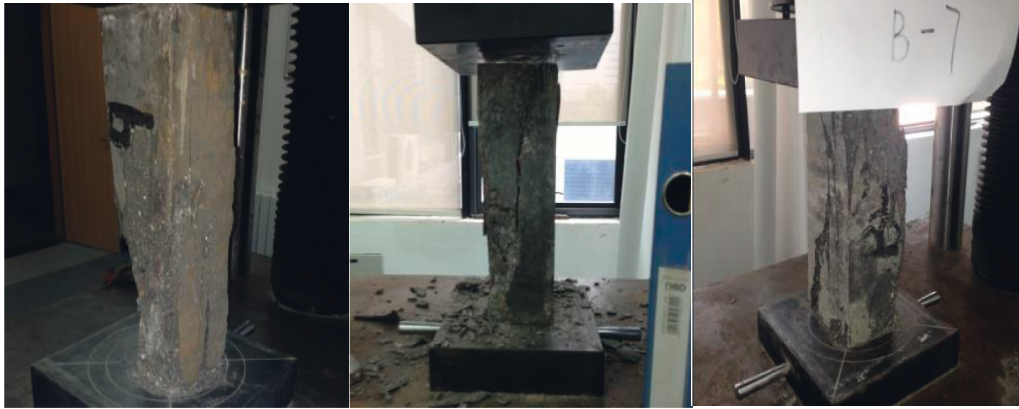
FIGURE 2: Shear failure as the major failure mode of prism specimens.
