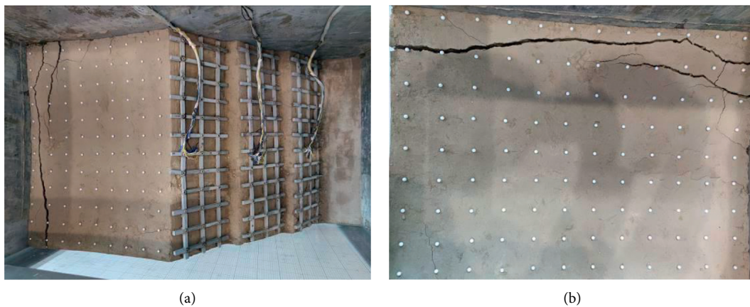
FIGURE 9: Slope deformation after test. (a) Overall deformation diagram of slope. (b) Partial diagram of slope top crack.
