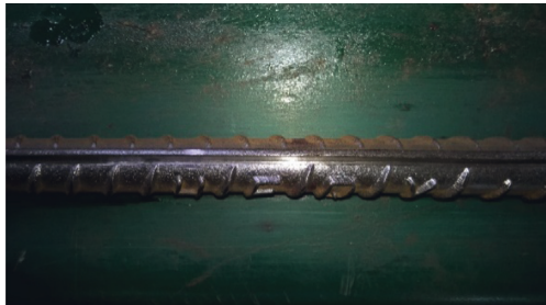
FIGURE 5: A groove of longitudinal reinforcement.
