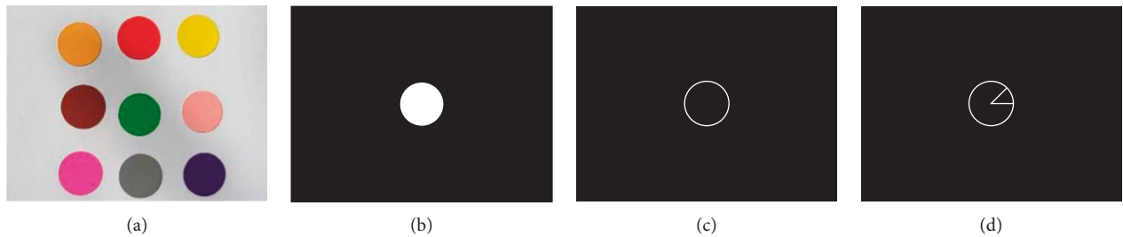
FIGURE 5: Algorithm detection effect. (a) The original image. (b) Color extraction in HSV. (c) Edge detection. (d) Hough's circle detection.
