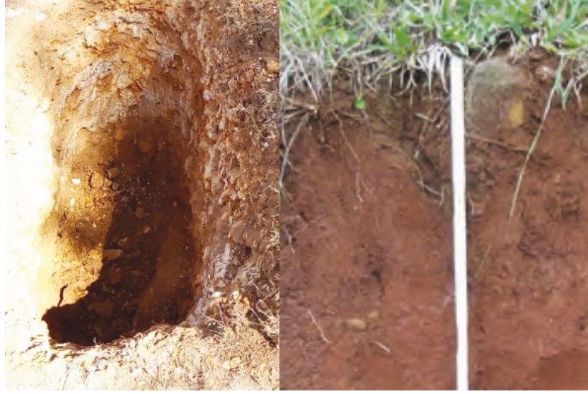
FIGURE 2: Test pit for a sampling of the soil.
