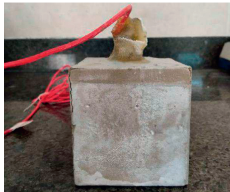
FIGURE 6: The cement soil sample cured using the seawater curing box.
