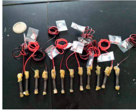
FIGURE 4: Steel bars after the anticorrosion treatment.
