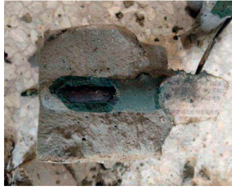
FIGURE 9: Removing the steel bar after breaking the cement soil sample.
