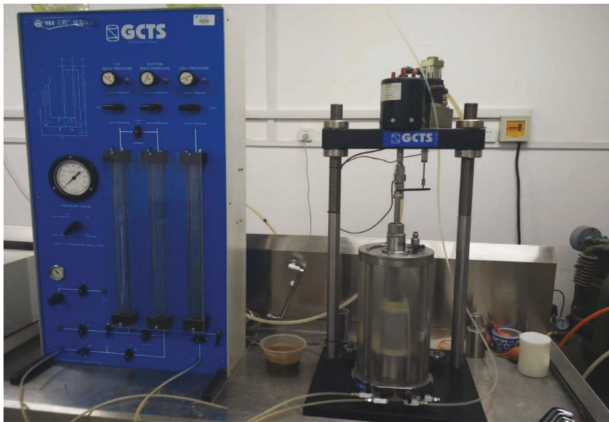
FIGURE 3: Dynamic triaxial test of sandy soil.
