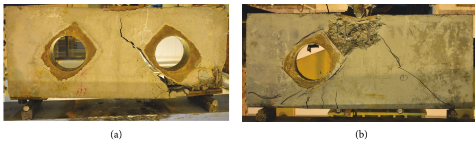
FIGURE 8: Failure modes of specimens strengthened with SPFs: (a) specimen S-F and (b) specimen E-F .
