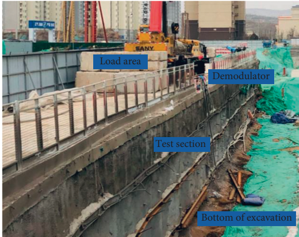
FIGURE 10: Arrangement of loading and unloading test.
