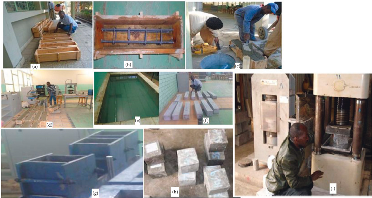
FIGURE 2: (a) Wooden formwork ready for casting, (b) wooden formwork with the steel cage, (c) mixing of concrete and compaction of beam samples, (d) compacting and placing of concrete in the mold, (e) keeping in water tank, (f) reinforced set of beam, (g) cubical molds, (h) cube sample, (i) compressive strength test.
