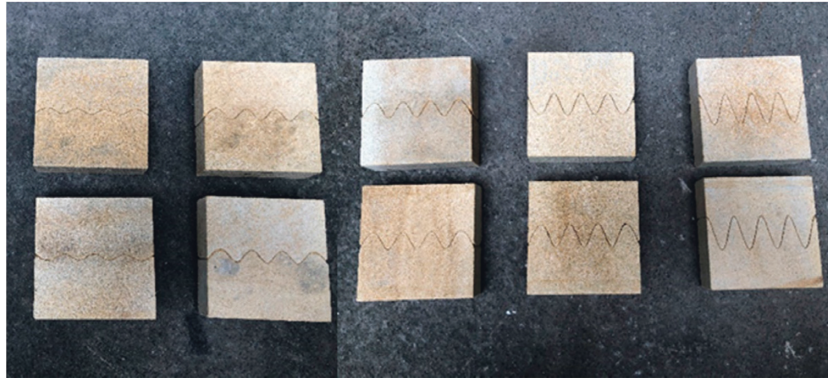
FIGURE 1: Specimens of fractures with different undulated heights.
