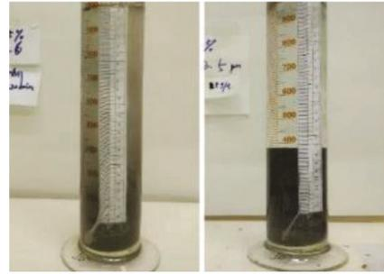
FIGURE 2: Comparison of natural settling and flocculation settling.
