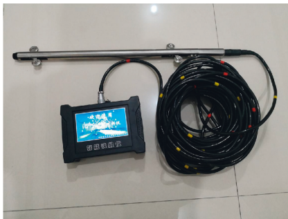
FIGURE 8: Photograph of the inclinometer used in engineering.
