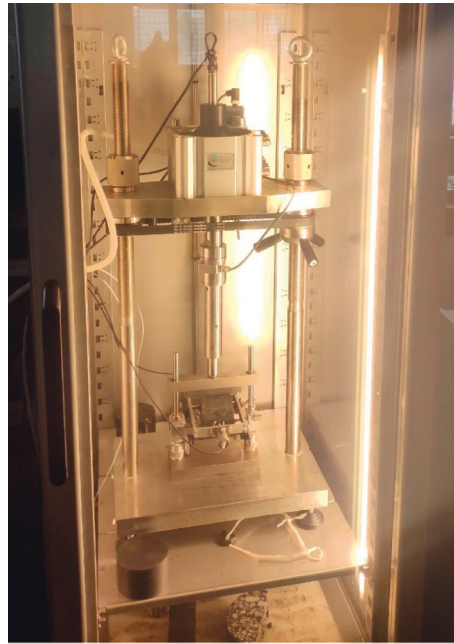
FIGURE 4: Resilient modulus test set-up.
