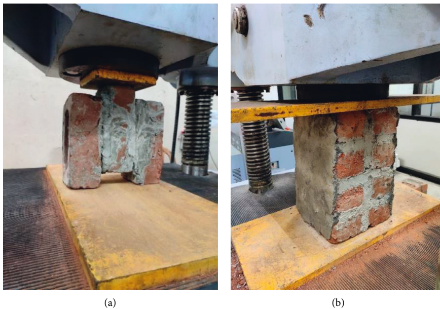
FIGURE 2: (a) Triplet test setup. (b) Specimen for compressive strength test.
