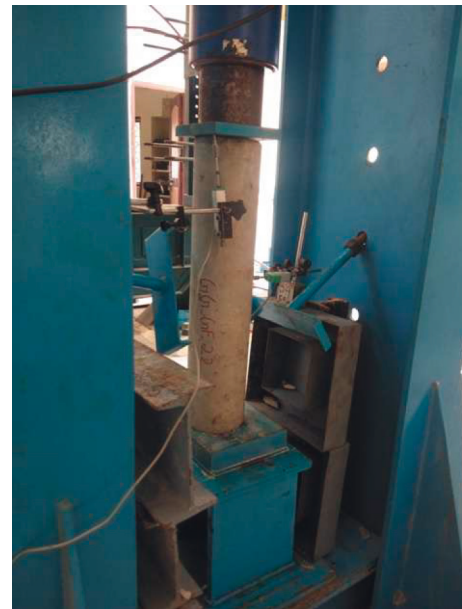
FIGURE 10: Test set up for axial loading.
