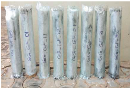
FIGURE 12: Column specimens wrapped with GFRP.
