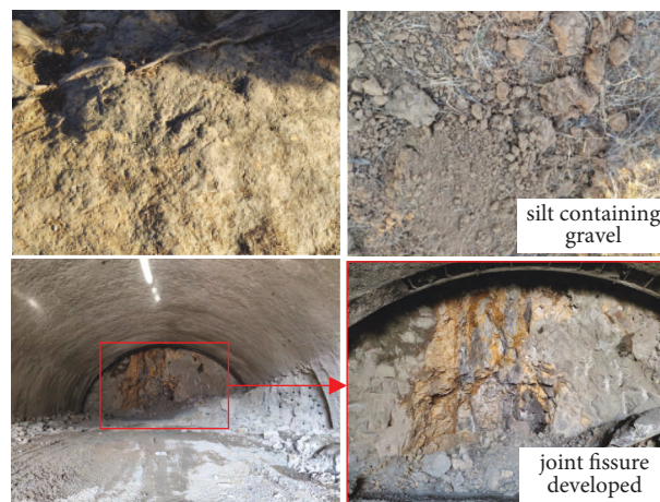
FIGURE 3: Geological features of surface residual soil and surrounding rock.
