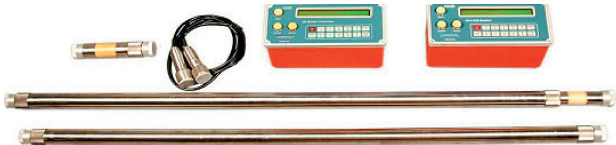
FIGURE 6: JW-6 underground high-frequency electromagnetic wave CT system.
