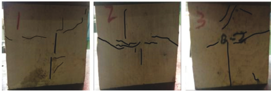
FIGURE 4: Failure mode of the specimen Y1.
