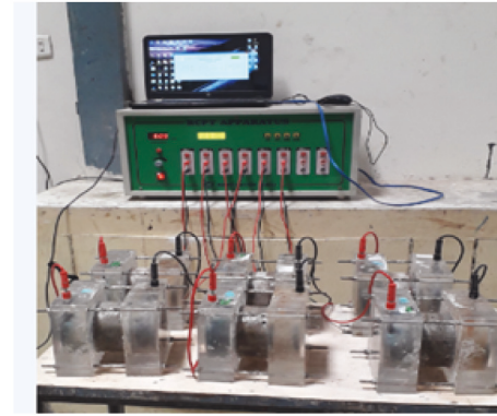
FIGURE 4: Test setup for RCPT test.
