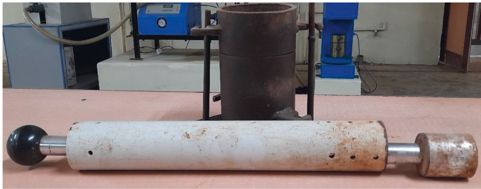
FIGURE 3: Set up for performing standard compaction tests.
