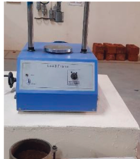
FIGURE 4: CBR test setup.
