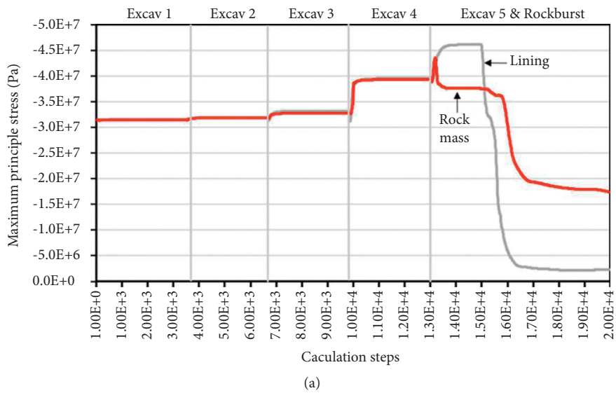
FIGURE 12: Simulation and comparison of rockburst disasters (discontinuous model): (a) weak support stiffness; (b) strong support stiffness.
