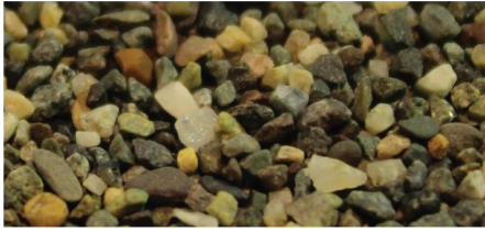
FIGURE 1: Example of flat angular sand particles.
