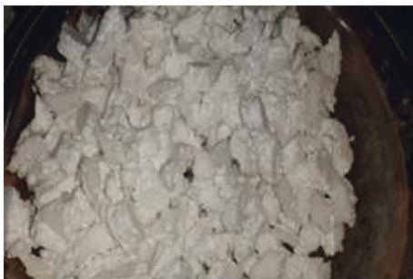
FIGURE 2: Shredded waste expanded polystyrene.
