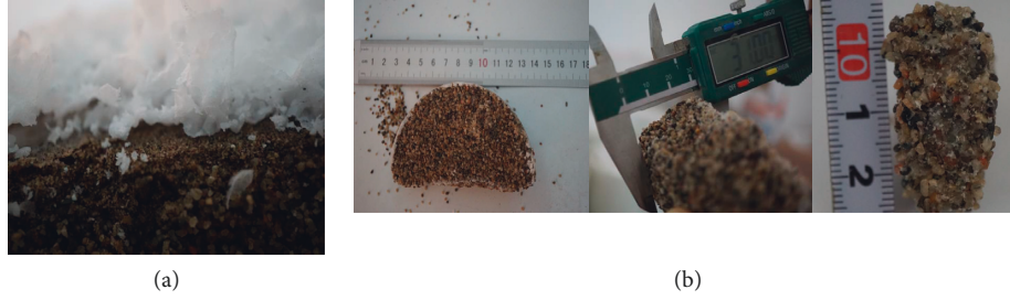
FIGURE 6: Heterogeneous column after the experiment. (a) The salt crust was elevated and formed salt domes. (b) The salt precipitated below the surface of coarse sand.
