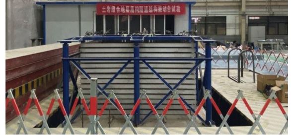
FIGURE 5: Shaking-table testing system.
