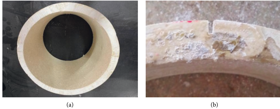
FIGURE 6: The slotted model of shield tunnel, (a) model pipe casting and forming, and (b) model pipe piece slotting.
