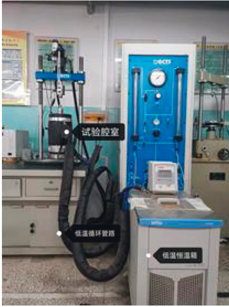
FIGURE 1: The STX-100 dynamic triaxial tester.
