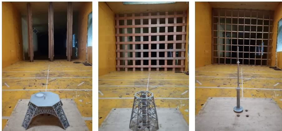
FIGURE 4: Images of the sectional model of the tower in the wind tunnel.
