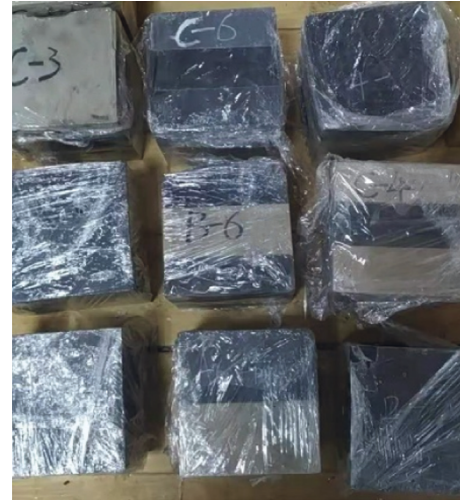
FIGURE 1: Coal-gangue interbed specimens.
