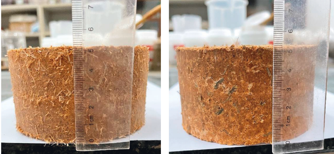
FIGURE 3: Reinforced glass fiber soil sample and reinforced basalt fiber soil sample.
