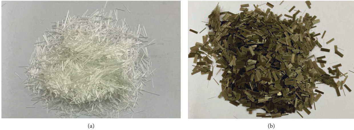
FIGURE 2: Material diagram. (a) Glass fiber. (b) Basalt fiber.
