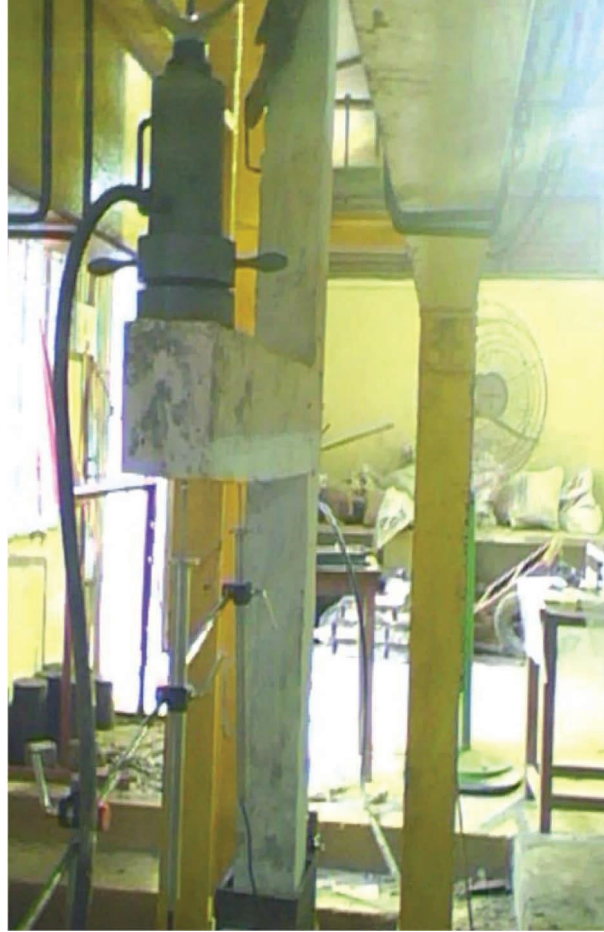
FIGURE 4: Actual test set-up on beam column joint under axial compression and flexure.
