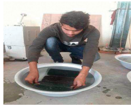
FIGURE 7: Water absorption test.
