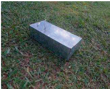
FIGURE 6: Mould prepared for the casting of bricks.
