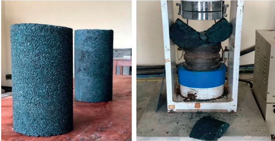
FIGURE 11: Split tensile test of plastic sand bricks.
