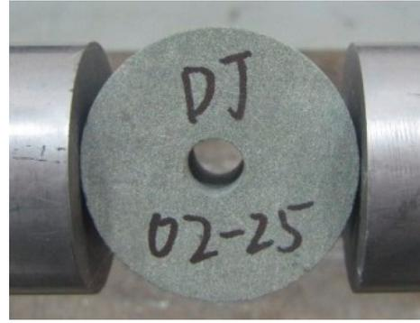
FIGURE 1: The clamping state of specimens.
