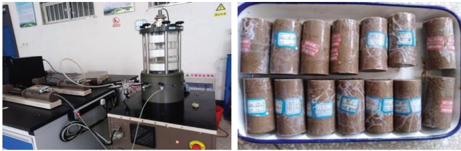
FIGURE 1: Dynamic triaxial testing apparatus and some W - D cycle samples.
