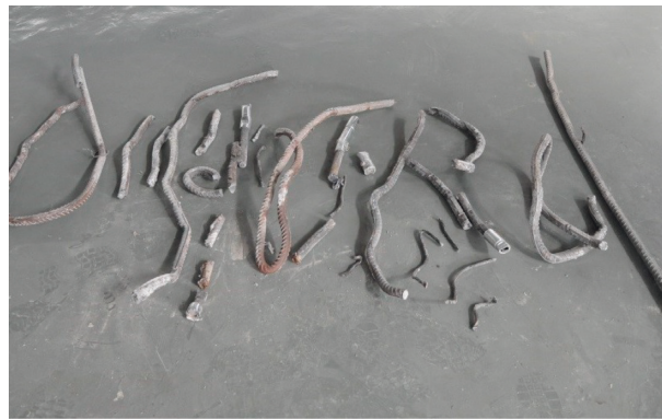
FIGURE 13: Rebars in the reinforced concrete cut by the cutters.
