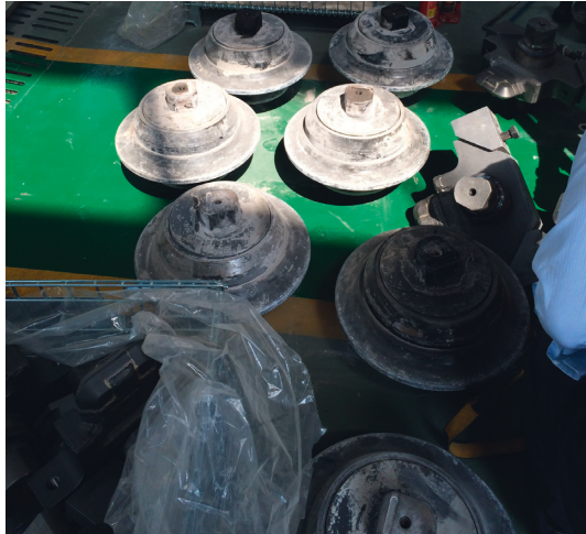
FIGURE 16: Cutters after test.
