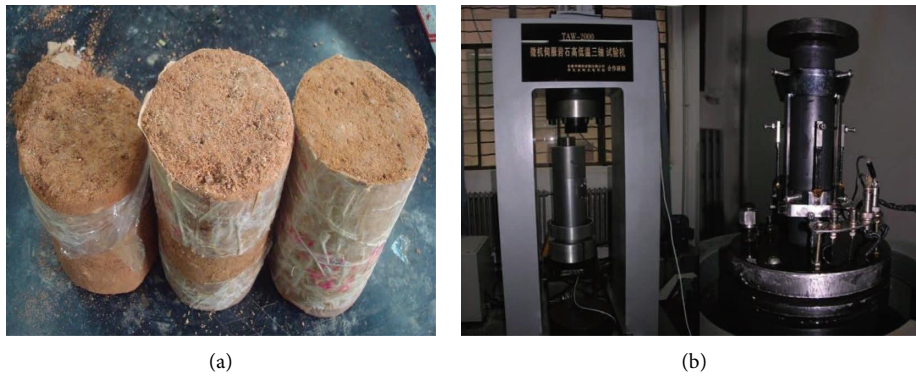
FIGURE 2: Rock mechanics test. (a) Sample sampling; (b) TAW-2000 microcomputer-controlled rock servo triaxial pressure testing machine.
