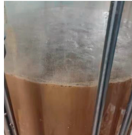
FIGURE 8: Bubbles generated from vacuum-saturated silt slurry.
