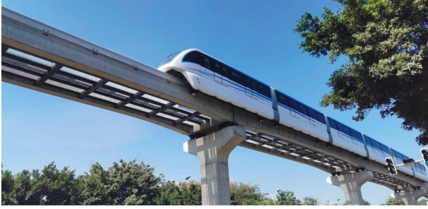
FIGURE 1: The transportation mode of straddle monorail is that the vehicle runs in the state of hugging the track.
