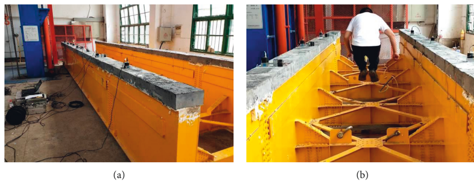
FIGURE 7: Dynamic test scheme. (a) Layout of vibration pickups. (b) Excitation scheme of person-jumping.
