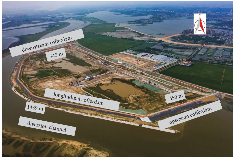
FIGURE 1: Layout of cofferdam and divert.
